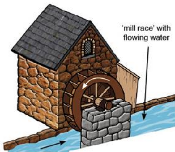
Example of an 'undershot' Water Wheel
