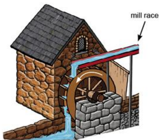
Example of a 'overshot' water wheel
